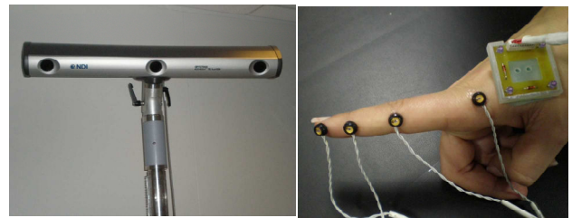
Fig. 10. OPTOTRAK Certus system and the experimental set-up.
