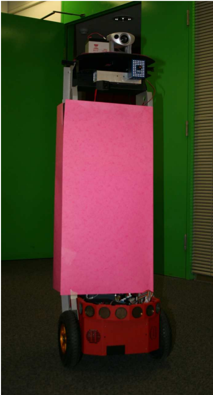
Fig. 3. The Peoplebot Robot. Note the luminous skirting for background segmentation as well as the time of flight camera, used for navigation, mounted at the top of the robot.
