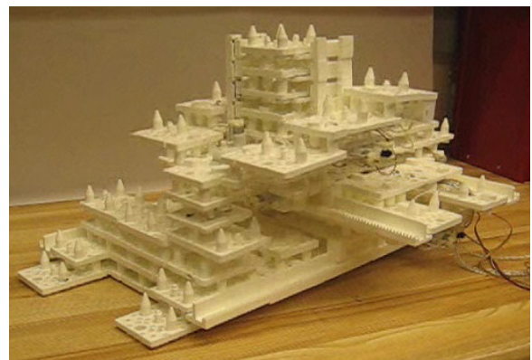
Fig. 12. A 3-axis Cartesian manipulator performs a demonstration task of stacking three modules, then removing them from the assembly station.
