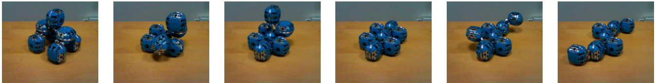
Fig. 6. Self-reconfiguration from car to snake; the self-reconfiguration process subsequently reverses and returns the robot to the car shape (not shown)
