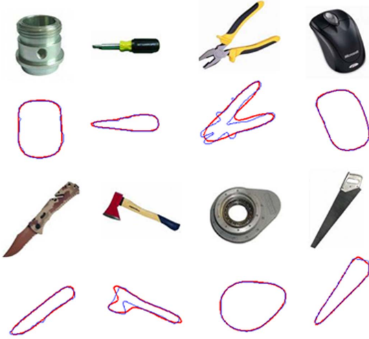
Fig. 1. Some sample objects and their outline curves obtained by regularized 3L fitting algorithm.
