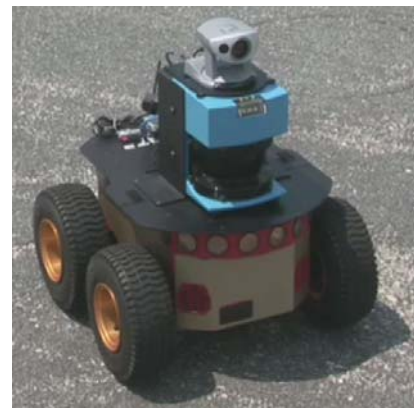
Fig. 8. Platform used for our first implementation of a Human-Robot Team Navigation System. The robot is a Pioneer 3AT from Mobile Robots, equipped with a pan-tilt camera and a laser range sensor.
