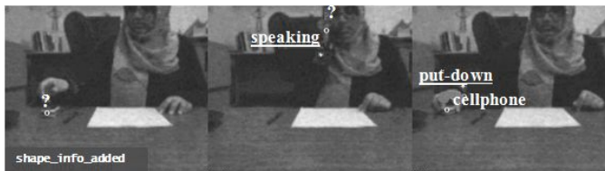
Fig. 11. Recognition results for the cellphone. Results of the object recognition algorithm are given as labels embedded on to each frame of the video. Video is taken from the left-eye camera of a QRIO robot.
