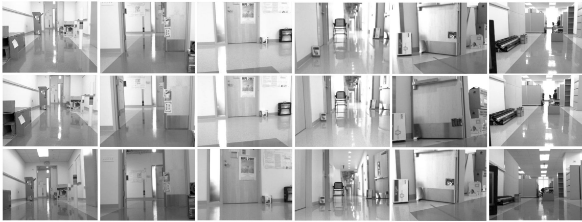
Fig. 8. With reference to Fig. 7, the top row shows the images collected while building the appearance map. Then middle row shows the corresponding view of the P3AT robot upon reaching those waypoints, while the bottom row shows the corresponding views for the iRobot Create.
