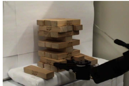
(e) The previous extraction attempt exceeded the movement threshold. A new block is selected.
