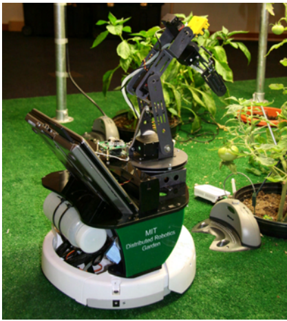
Fig. 2. Robots are equipped with an end-effector, camera, localization system and watering device that are controlled by a notebook computer. Plants are enhanced with a wireless embedded Linux device that can monitor its status using a humidity sensor and information collected by the robot as well as issue requests.
