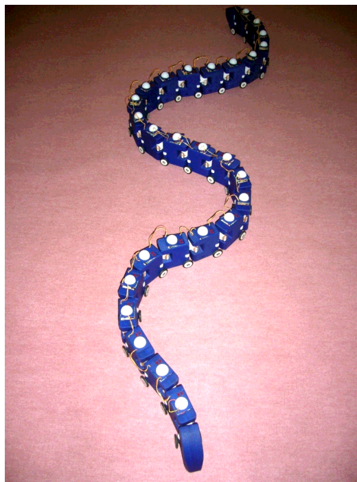
Fig. 6. A whole image of the 2D serpentine robot developed.
