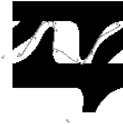
Fig. 5. Configuration space of the 2R manipulator. The white region shows the free space. The black squares show configurations along the collision-free trajectory. The positions of the manipulator in the workspace corresponding to the configurations are shown in Figures 9 and 10. The points S and G are the start and goal configurations respectively.
