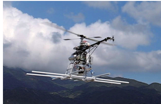
Fig. 1. The instrumented JR Voyager GSR 260 under the governance of the proposed controller. The white bars below the landing gear were installed to avoid flapping during touch-down.
