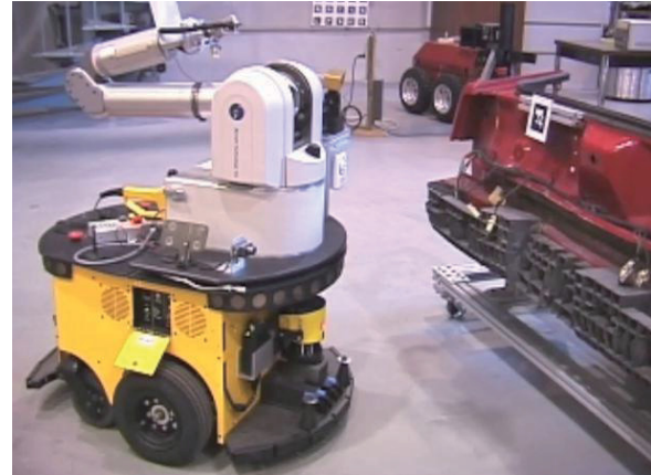
Figure 1. Our mobile manipulator consists of a PowerBot mobile base with a 7-DOF WAM arm, a Bumblebee stereo camera mounted on a pan-tilt unit, and a SICK laser scanner. Also shown is the task board with a visual fiducial marker used for pose estimation.
