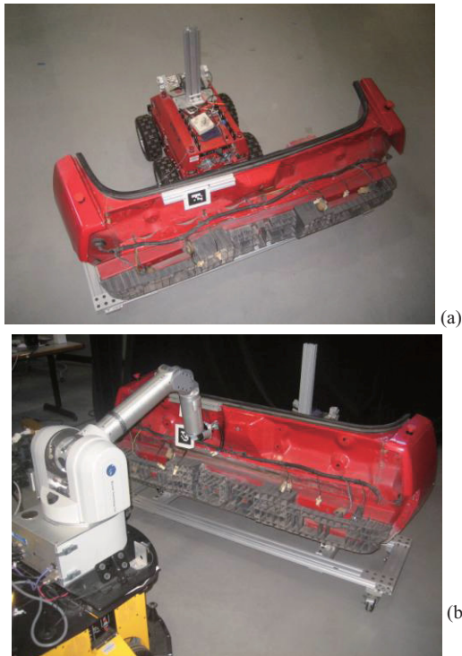
Figure 11. (a) An ATRV-Jr. robot is commanded to move the task board at a constant speed. (b) The WAM arm end-effector keeps contact while the mobile base is tracking the task board movement using a pure pursuit algorithm with a low pass filter.
