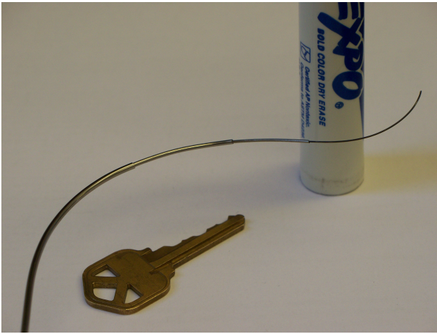
Fig. 2. An active cannula with 4 concentric tubes. Each concentric tube is pre-shaped with a different radius of curvature, with the thinner, inner tubes having higher curvature.
