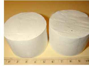
Fig. 3. The left and right cylindrical specimens are “hard” and “soft” silicone, respectively. The dimensions of both specimens are 25mm in radius and 30mm in height.
