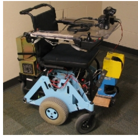
Fig. 5: The wheelchair robot used for collecting the video datasets. The robot has a stereo camera and one horizontal and one vertical laser-rangefinder. The lasers are only used for localization and providing ground truth data.
