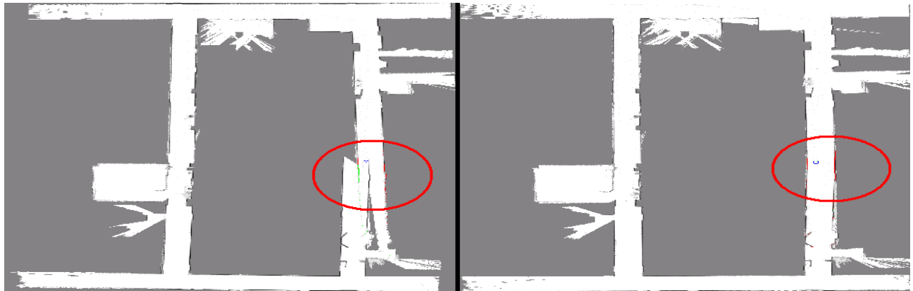
Fig. 4 SLAM in the CSIE building with general approach (left), and hybrid approach(right).
