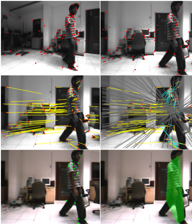
Fig. 5. TOP LEFT: An image with stationary objects and a moving person as the P3DX rotates while translating. The KLT features are shown in red. TOP RIGHT: A subsequent image after further rotation and translation MIDDLE LEFT: The flow vectors shown in yellow. MIDDLE RIGHT: Flow vectors in yellow, epipolar lines in gray and perpendicular distances in cyan. BOTTOM LEFT: Features classified as dynamic, shown in green. BOTTOM RIGHT: Convex hull in green overlaid over motion regions.
