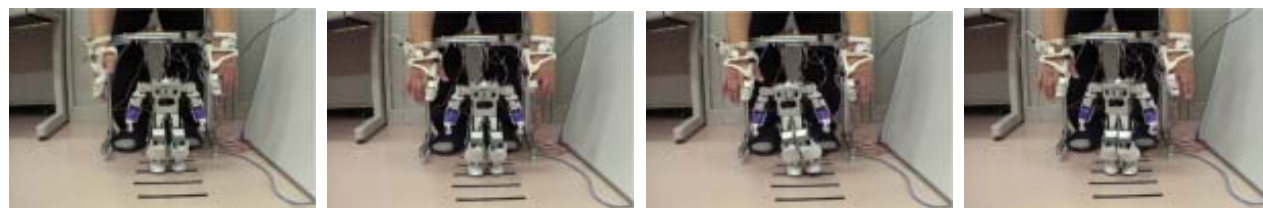
(a) Walking direction set by right forearm's supination (b) Flexion of index finger of left hand (c) COM Shift to right side for 1st rotation (d) 1st rotation (Left leg has just landed.)
