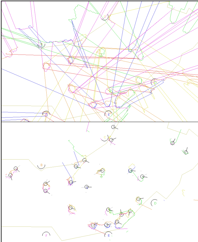
Figure 2. Scan data from six laser range finders in our field trial space on a busy day. (Top) Raw laser scan data. (Bottom) Scan after processing and background removal, including locations of detected people.
