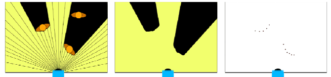
Figure 5: A typical single-sensor laser scan. (Left) The positions of humans relative to the scanner. (Center) Occupancy information. (Right) Edge information.
