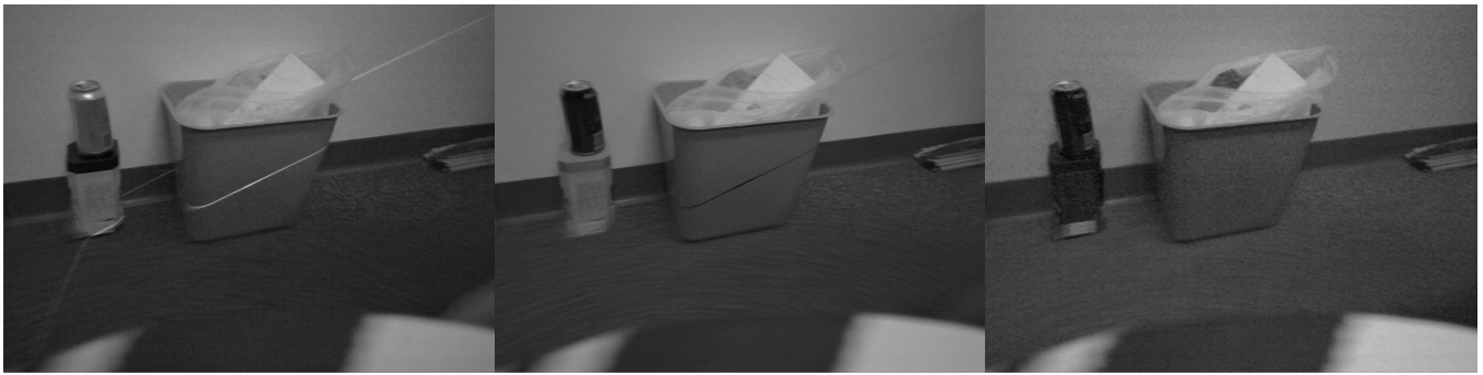
Fig. 4. RGB colour components of single image illustrating how the red laser line is still slightly apparent in the green component but not the blue.
