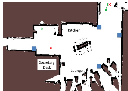
Fig. 1. A hindrance-sensitive robot path planning problem in our experimental environment containing a person (green square) in the upper right with a previous trajectory (green line) and intended destination (green X) near a doorway, and a robot (red square) near the secretary desk with its intended destination (red X) near the person’s starting location. Hindrances are likely if the person and robot both take the distance-minimizing path to their intended destinations. Laser scanners are denoted with blue boxes.
