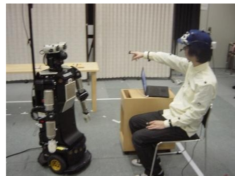
Fig. 14 Robot system for recognizing a referred-to object.
