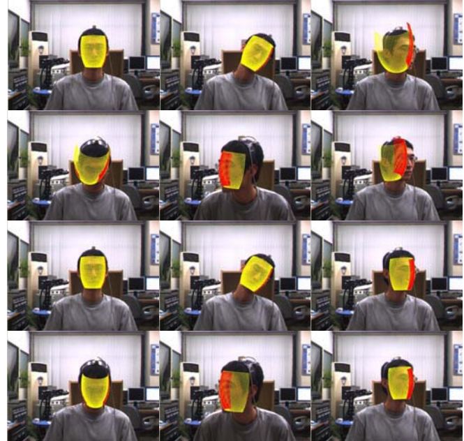
Fig. 4. Typical tracking results on one of the sequences taken under near-uniform illumination. Frames 1, 55, 112, 164, 193, and 300 are shown (left to right, top to bottom). Rows 1~2: conventional method without illumination correction; Rows 3~4: our proposed unified method including illumination correction.
