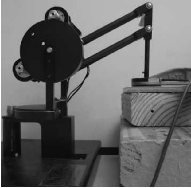
Fig. 4. EXPERIMENTAL SETUP: BOTH THE PHANTOM AND FORCE SENSOR ARE FIXED TO THE TABLE. THE DIRECTION OF STATIC FORCES IS MEASURED.
