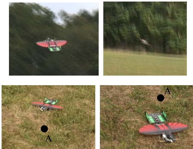
Fig. 14. Upper-left: MALV 2 climbs to cruising altitude after hand launch. Upper-right: MALV 2 approaches for a landing. Lower left: MALV 2 at the landing point. Lower-right: MALV 2 crawling away from the landing point. The dot ‘A’ is stationary with respect to ground.
