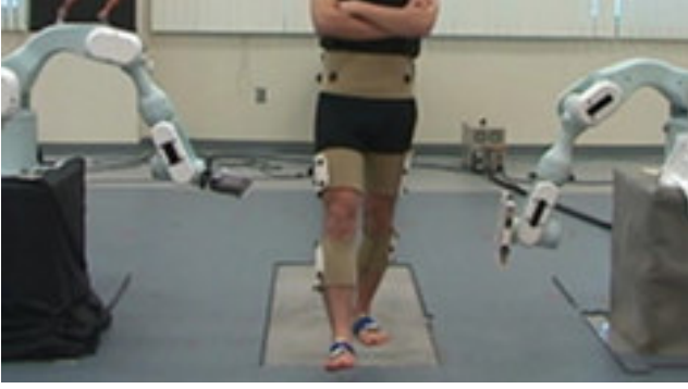
Figure 1. Prototype imaging platform that will be used for dynamic X-ray imaging as well as cone-beam computed tomography and traditional imaging tasks.
