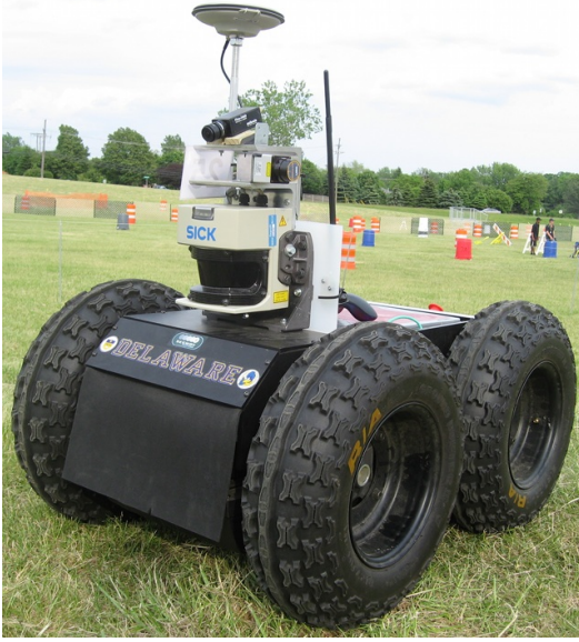
Fig. 2. “Warthog”: Segway RMP 400 robot platform with color camera, SICK lidar, and sagittally-mounted Hokuyo URG
