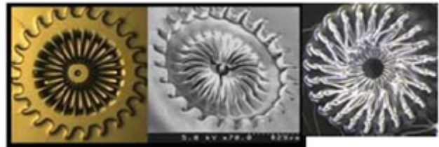
Fig. 7: Three-dimensional patterning of KMPR
