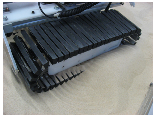
Fig.16: Infiltration of Sand into the Conventional Tracked Belt
