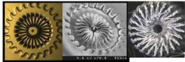
Fig.7: Three-dimensional patterning of KMPR
