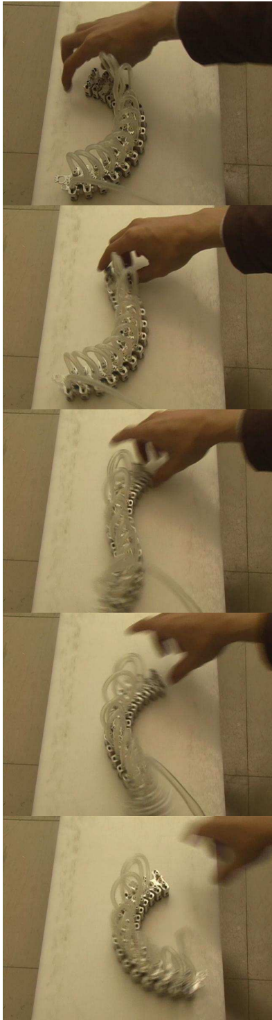
Fig. 9. Motion without lateral constraints: The head unit is manually turned right and the body rapidly change its shape from mirrored C-shape to C-shape
