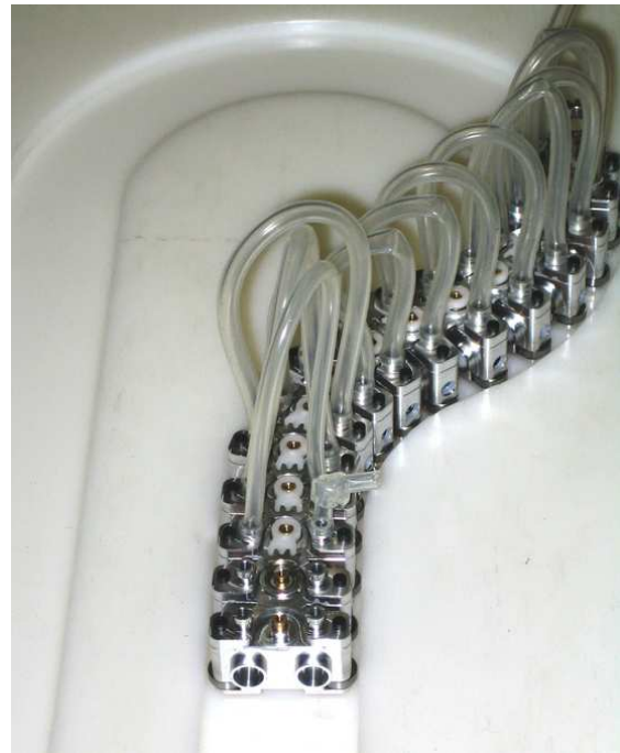
Fig. 6. Front view of partly assembled prototype; 15 units are joined. The first two units are used as a "steering", so no air pressure is supplied.
