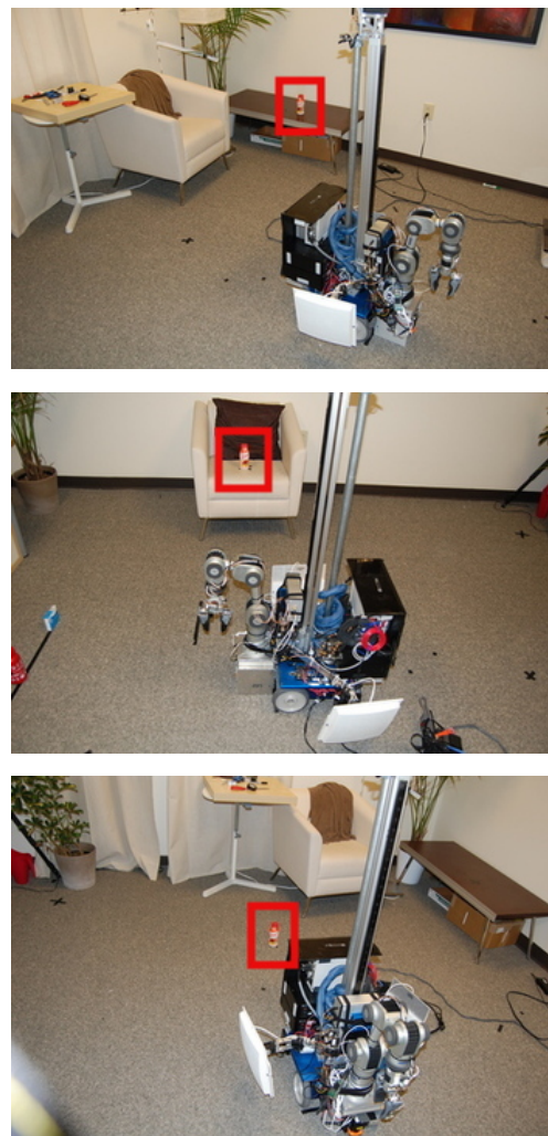
Fig. 10. Three different bearing estimation scenarios, with object locations highlighted. Bearing estimation was attempted for all three objects, each in the three different locations (9 total attempts). In 8 of 9 instances, the robot correctly achieved a bearing that placed the tagged object in the fused sensor image.
