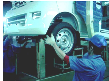
Figure 1 The current manual wheel loading process. Typically there are 6 operators per shift and two shifts per day.
