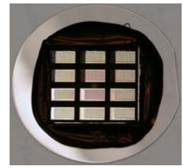
Fig. 4. The tubes are embedded in the wax (black) after the backing Si is etched.
