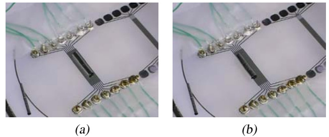
Fig. 15. The tube in motion. a) tube moving forward, b) tube moving backward. The video can be found at Http://www.cs.cmu.edu/~claytronics/movies/1x_tube_back-and-forth.mp4 .
