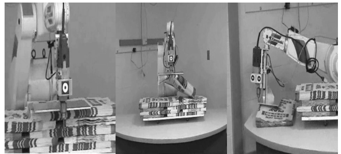
Fig. 15 The robot inserted the tool into the gap and pick up the bags
