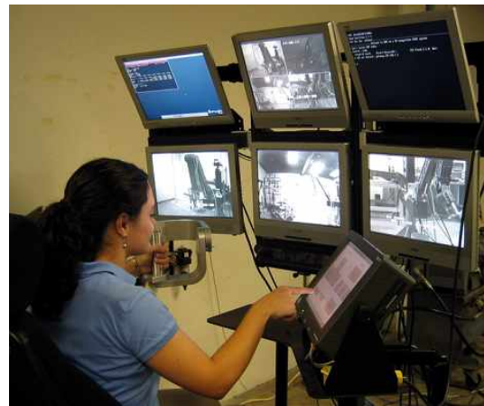
Figure 2. The operator controlling the arm and the gripper from the CRC using the WAM.
