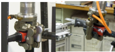
Figure 8. Cutting aluminum rod and steel pipe
