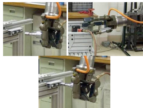
Figure 9. Removing a bolt using an impact wrench
