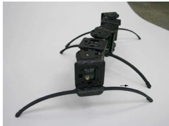
Fig. 6. Dynamic centipede with springy legs for jumping[11]
