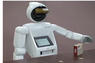
Fig. 1. A shot from an on-line experiment with object detection and pose estimation on our robot platform, Enon. The robot was about to grab the object after estimating its pose successfully.
