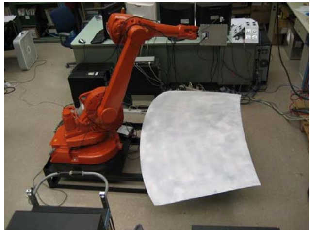
Fig. 12. Automatic 3D Rapid Windshield Inspection System
