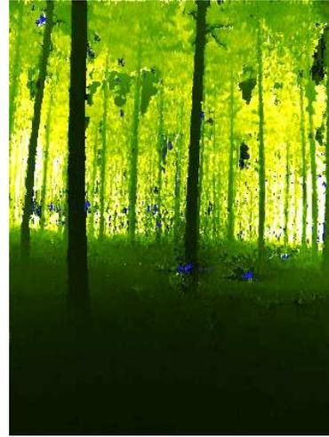
Fig. 4. Depth map corresponding to an image pair. The brighter the color, the more distant the image location is. Due to the scale invariance, the depth map information is relative.
