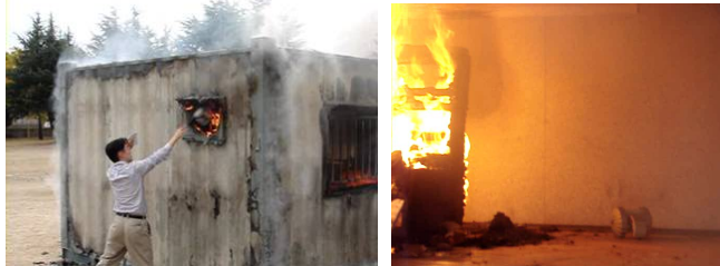
Fig. 11. Experiments with fire in container house
