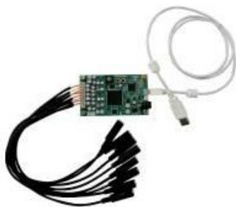
Fig. 3. 8 Channel A/D converter board with microphone cables
