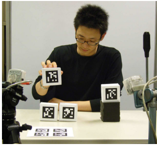
Fig. 1. System overview. Two cameras are pointing down to a desk and observing a human instructor demonstrating a task. Physical synthetic markers are applied on objects and placed on a desk to estimate pose of cameras and objects.
