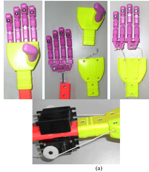
Fig.8 Rock-Scissors-Paper Prosthetic Hand. (a) Appearance. (b) The DOF diagram of the hand part.
