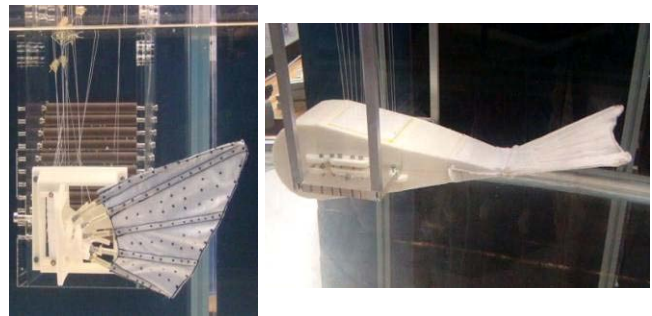
Fig.1. Biorobotic pectoral (left) and caudal (right) fins.
