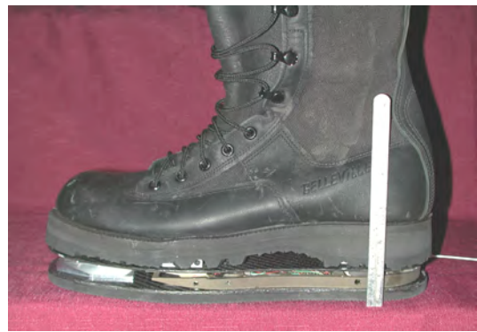
Fig. 1. Foot force-torque sensor attached to boot.
