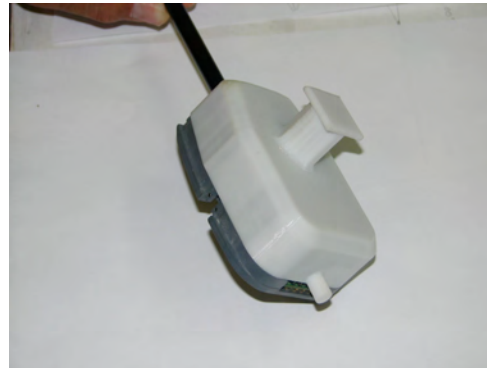
Fig. 4. Modified tool cover for robust end-effector grasping.
