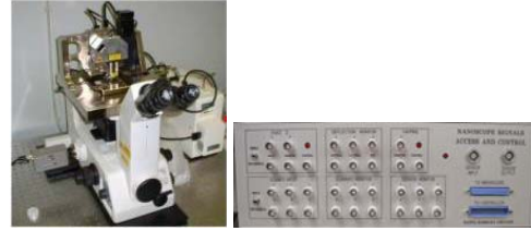
Fig. 5. The AFM system and the signal access module.
